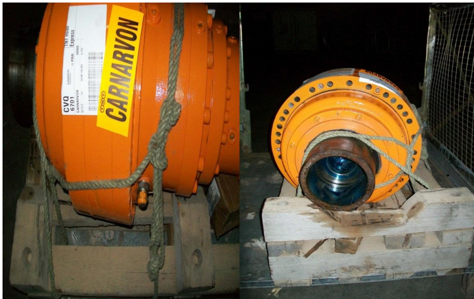
Rope is not to be used to secure freight
