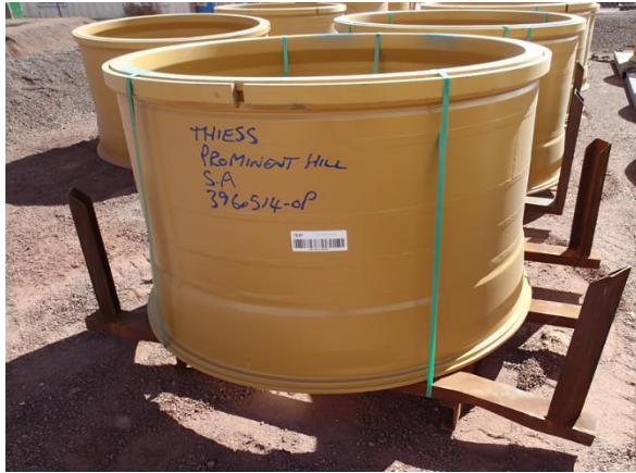
OTR Wheel Rims inadequately restrained, unsecure dunnage, potential for metal on metal slippage.
