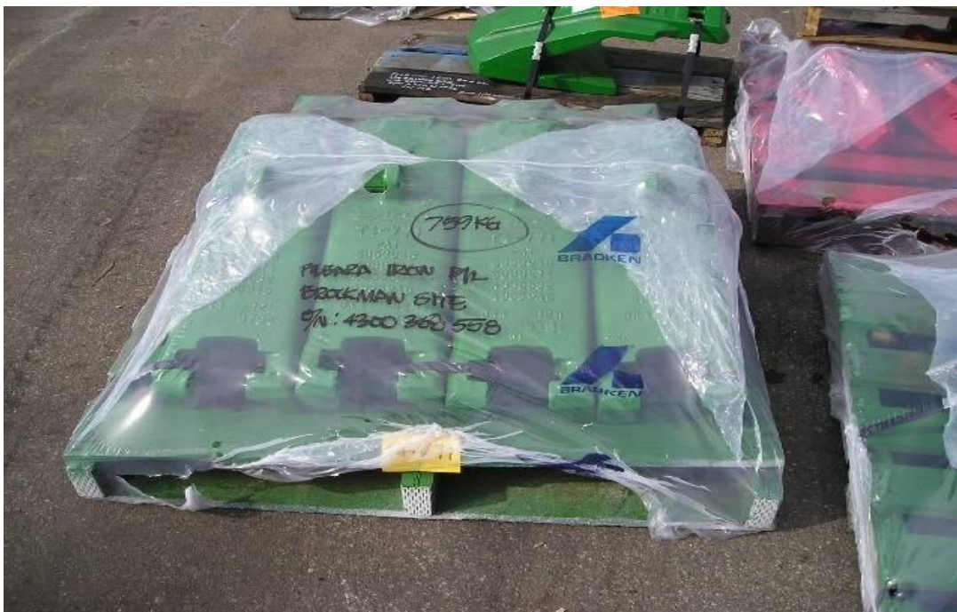
A well packaged consignment on a good sturdy pallet. Metal banding is under the bearers
