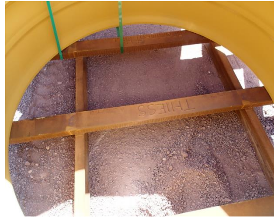
OTR Wheel Rims inadequately restrained, unsecure dunnage, potential for metal on metal slippage.
